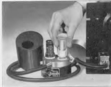
Figure 5. View of pre-amplifier and quenching circuit assembly with cover removed to show Type 1500-P2 Beta-Ray Counter. Note the convenient arrangement for plugging in the counter tube.
