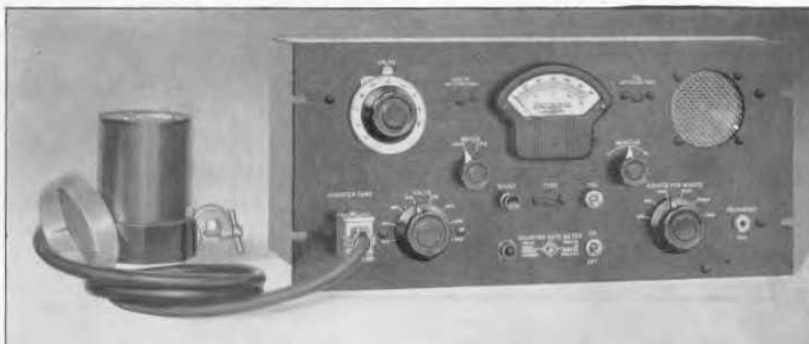
Figure 1 Panel view of the Type 1500-A Counting-Rate Meter with counter tube plugged in.
